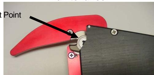
Lubricate the AxelCut Blades pivot point with one or two drops of light turbine oil or equivalent on a semi-annual basis. **Important: Do not use solvents on the blades.**
