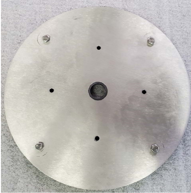
Figure 4 Top Plate with Bushing Installed
