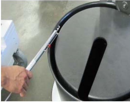
Figure 7 Checking Rotatub Slip Value
