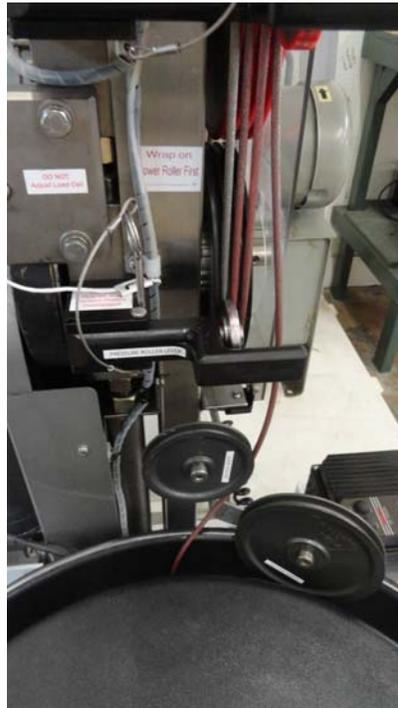
Remember, the clutch can slip and slow down the Rotatub, but it cannot increase the Rotatub speed if the Pitch diameter of the cable coming off the capstans is too large and the clutch is adjusted properly.
