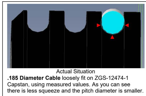
**Effect of Cable Load:** The higher the load the further the cable gets pulled down into the grooves of the capstans; therefore, the pitch diameter is reduced and the cable comes off the capstans slower. Conversely the lower the load, the higher the cable rides in the groove; therefore, the greater the pitch diameter and the cable comes off the capstans at a higher speed.
