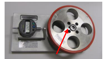
Insert capstan with keyway facing the indicator (shown is a 4-groove capstan)
