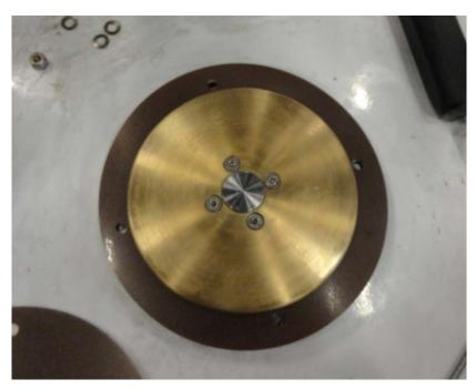
10. Place the next slip pad on top of the bronze disc and align the holes in the plate with the holes in the slip pads.
