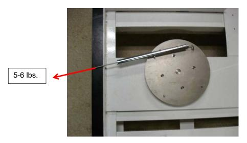
18. The final check is made with the Rotatub reattached to the platen. Use a spring scale to hold the tub while the extend switch is actuated. The force at the tangent to the tub edge should be 2 to 3 lbs. with the slip pads slipping.
