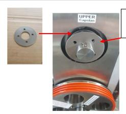
Step 2 Place spacer on shaft Align 4 through holes
