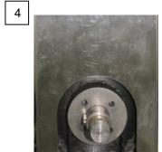
Remove the .8 Key and Spacer and set aside for reassembly This will leave the pulley exposed
