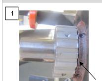
Verify the pulley is flush to the sprocket (If space is visible between pulley and sprocket proceed to next step)
