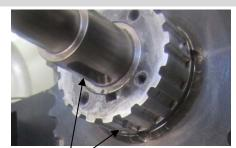
Tighten the set screw that is located directly in line with the key location
