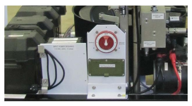
To use the onboard batteries, the switch should be in position 1, and to use the external power receptacle the switch should be in position 2.
