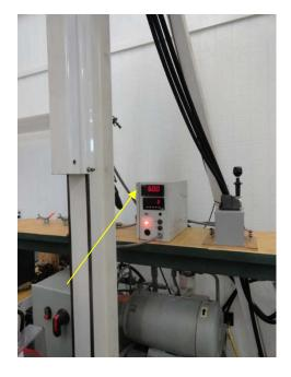
The position of the bolt is just right to apply a 600 lbs. load to the hook.
