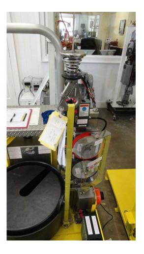
When the frame starts to lift off the ground, a load of 600 lbs. is applied to the cable via the hook.
