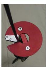
Verify the bitter end is captured as shown and the cable is behind the retainer in the top plate. The quick splice is ready for use. The hoist cable must be replaced upon completion of the mission.
