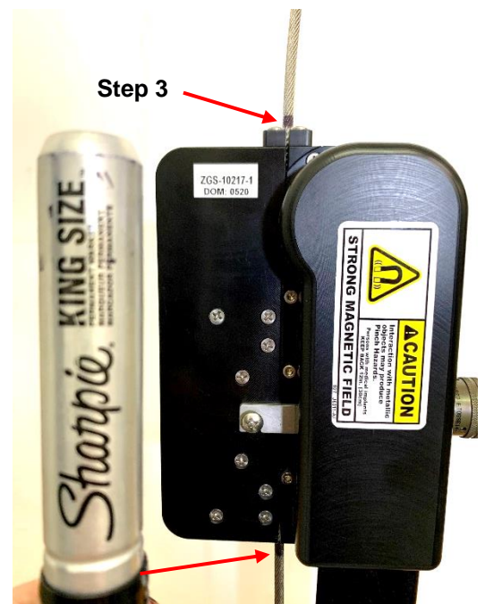
Figure 22 Marking cable for inspection
