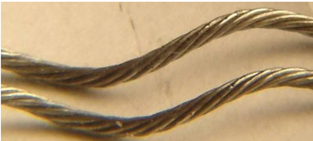
Figure 38 Severe internal peening
