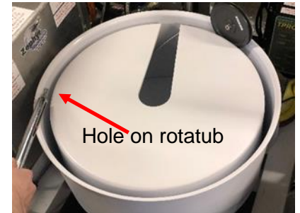
Figure 56 Quick Slip Load Check of Rotatub
