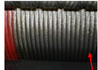
Maintains clean & tight Cable storage on the rescue hoist Brake Drum. Figure 4 RHGSE usage results in tight wraps
