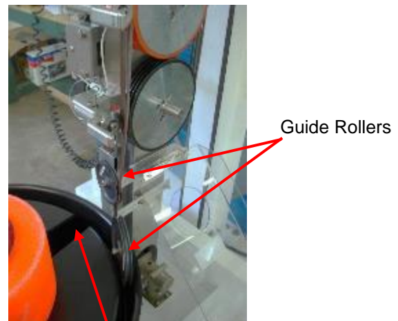
Figure 28 Proper cable positioning in Rotatub and Spooler
