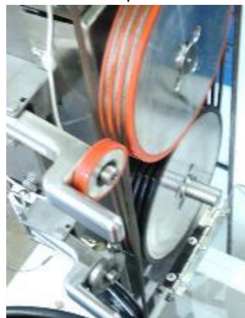
Wrap around the third groove
