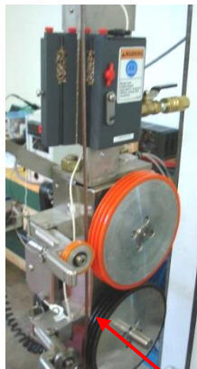
Start wrapping the cable in the first groove of the lower capstan
