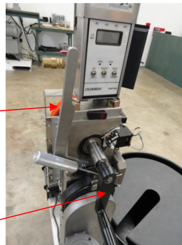
Shown is the load lever engaged and crank handle disengaged
