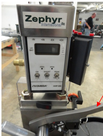
Shown is the load lever disengaged
