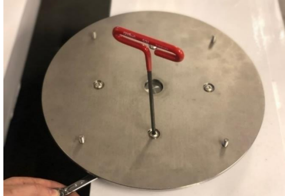
Figure 43 Adjusting clutch adjustment screws
