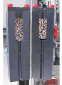
Figure 46 New Pads Installed
