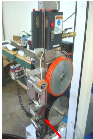
Start wrapping the cable in the first groove of the lower capstan
