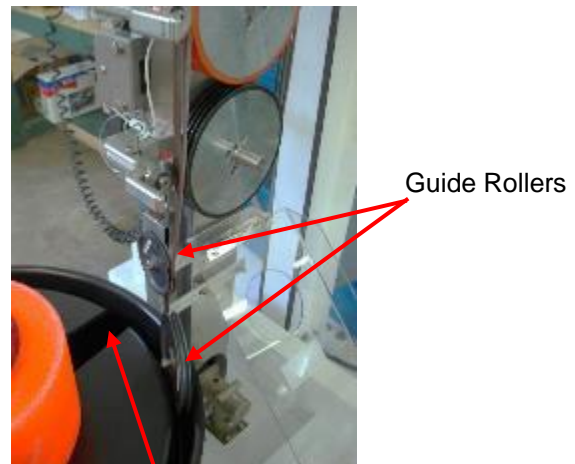
Figure 24 Proper cable positioning in Rotatub and Spooler
