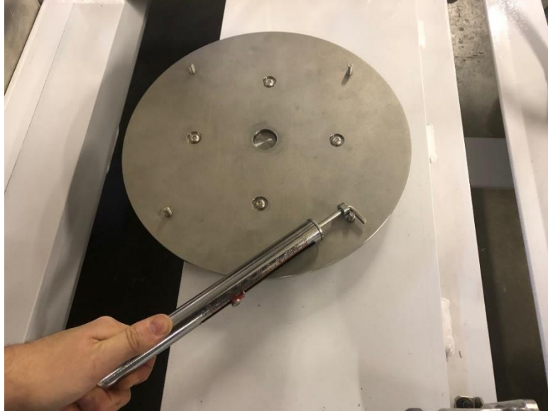
Figure 45 Measuring the Rotatub slip value
