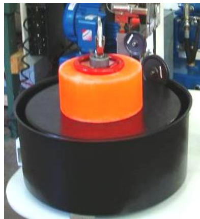
Figure 24 Proper cable positioning in Rotatub and Spooler
