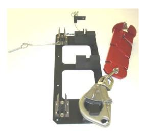
2) Place the hook attachment bolt head down into the center rubber pad and pull the QuickSplice plate up into the slot as far as it will go.
