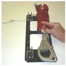
3) Place the retaining bracket into the slot of the QuickSplice. Pull the QuickSplice towards the top of the QuickSplice Mounting Bracket while inserting the locking pin through the retainer bracket and the QuickSplice Mounting Bracket.
