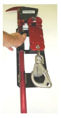
4) Insert the retaining pin into the upper bracket to lock the AxelCut into position.
