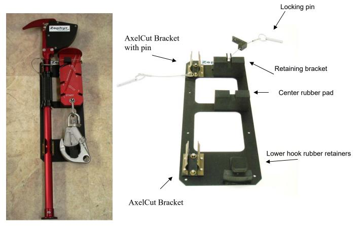
It is designed to hold the AxelCut and QuickSplice securely, yet allow their release quickly in an emergency.
