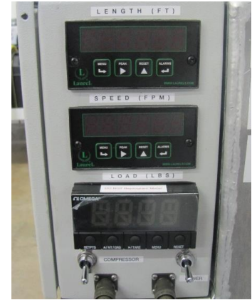
Figure 22 - Control Station - Digital Displays
