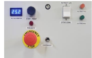
Figure 23 - Control Station - User Interface
