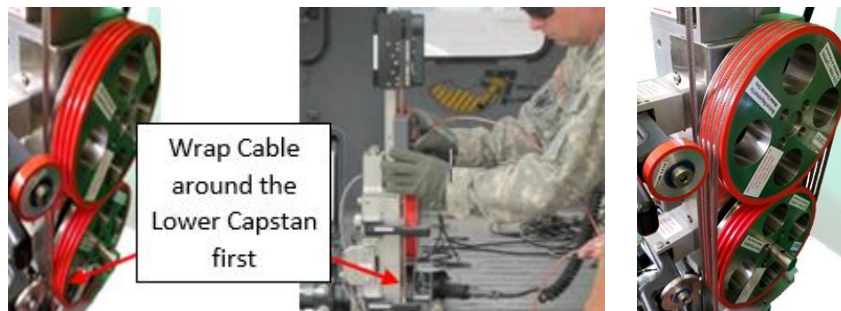
Figure 37 - Capstan Cable Wrap
